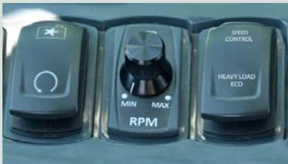
Finally, EPD Top includes the control of the engine revolutions proportionally to the use of the joystick (the greater the inclination of the joystick, the greater the engine revolutions). Functionality optimised for material handling.
